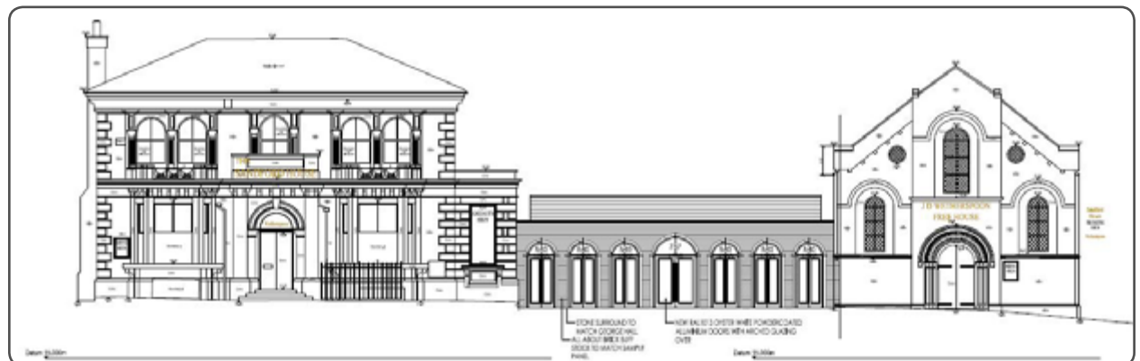
Front elevation of Sandford House, showing the extension linking the two old buildings
