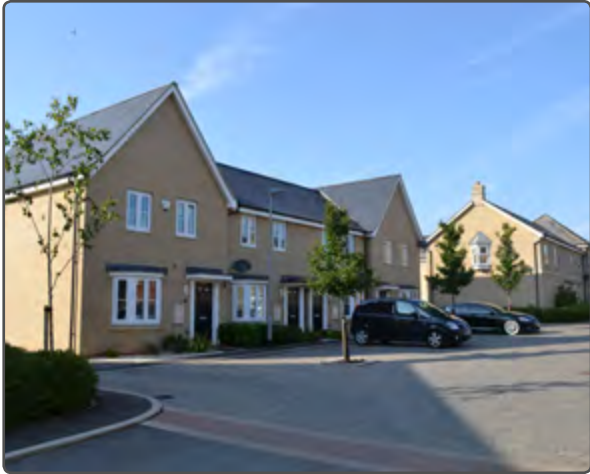
This informal car parking is made possible by widening the street and using trees - St Neots
