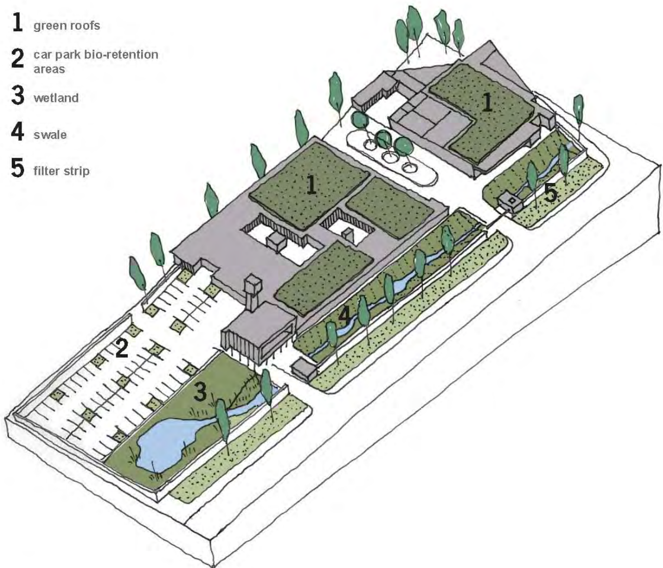
Figure 6.18 : Incorporating SuDS on industrial sites
