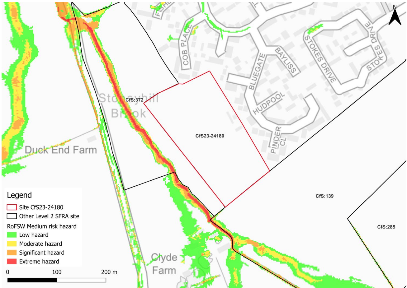
Figure 3-3: Medium risk event surface water flood hazard 1 (Third generation - Risk of Flooding from Surface Water map)
