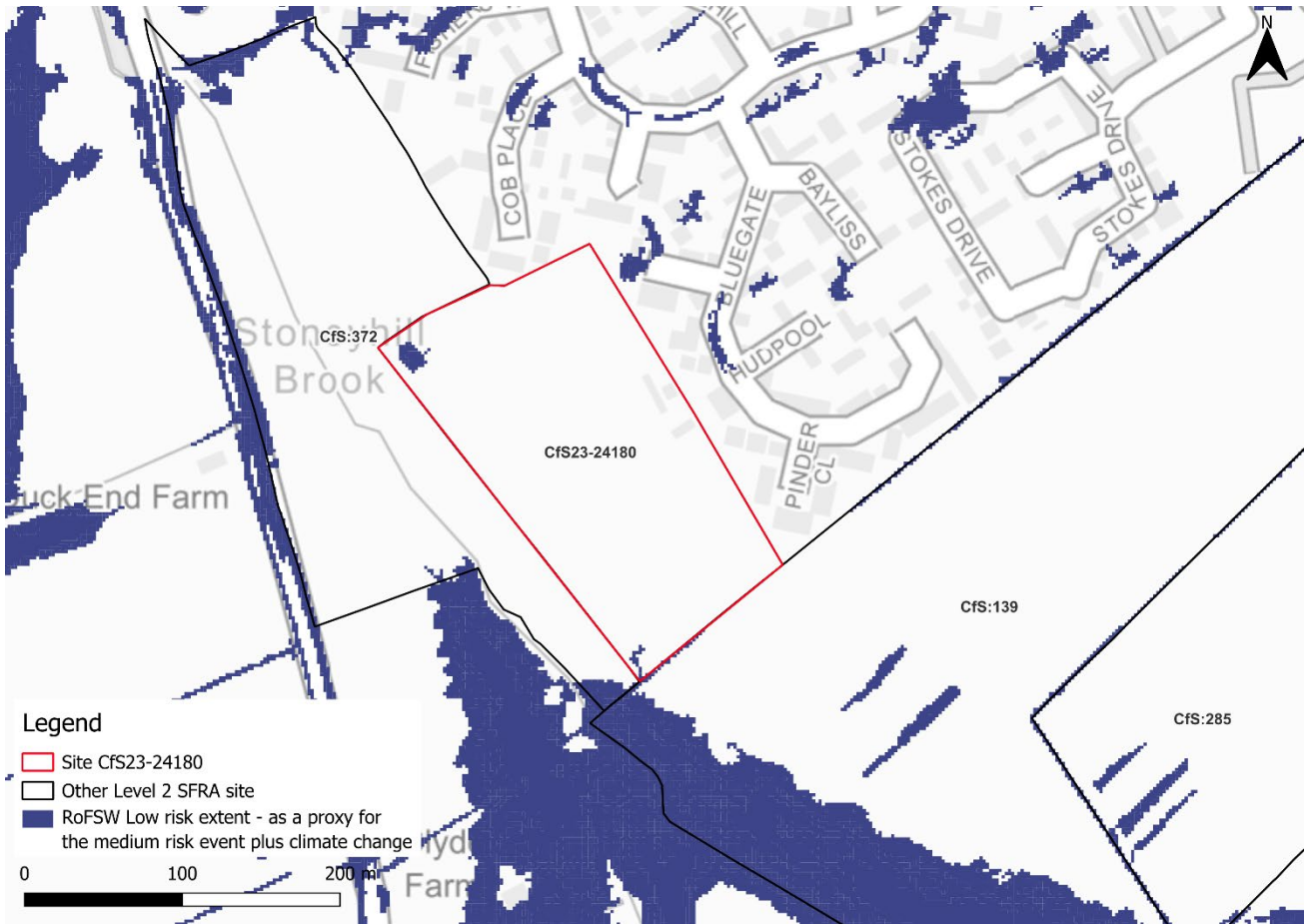
Figure 3-4: Low risk event surface water flood extent, as a proxy for the medium risk event plus climate change (NaFRA2 - Risk of Flooding from Surface Water map)
